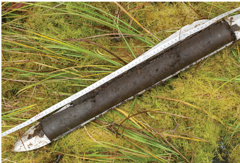
Figure 4. Drilling from the Březina peat-bog. Freshly sampled sediment core in boring chamber tool, basis of the profile. The grey part at the bottom corresponds to starting sedimentation at the beginning of the Holocene, followed by sedimentation of a woody fen. © Jindřich Prach.
