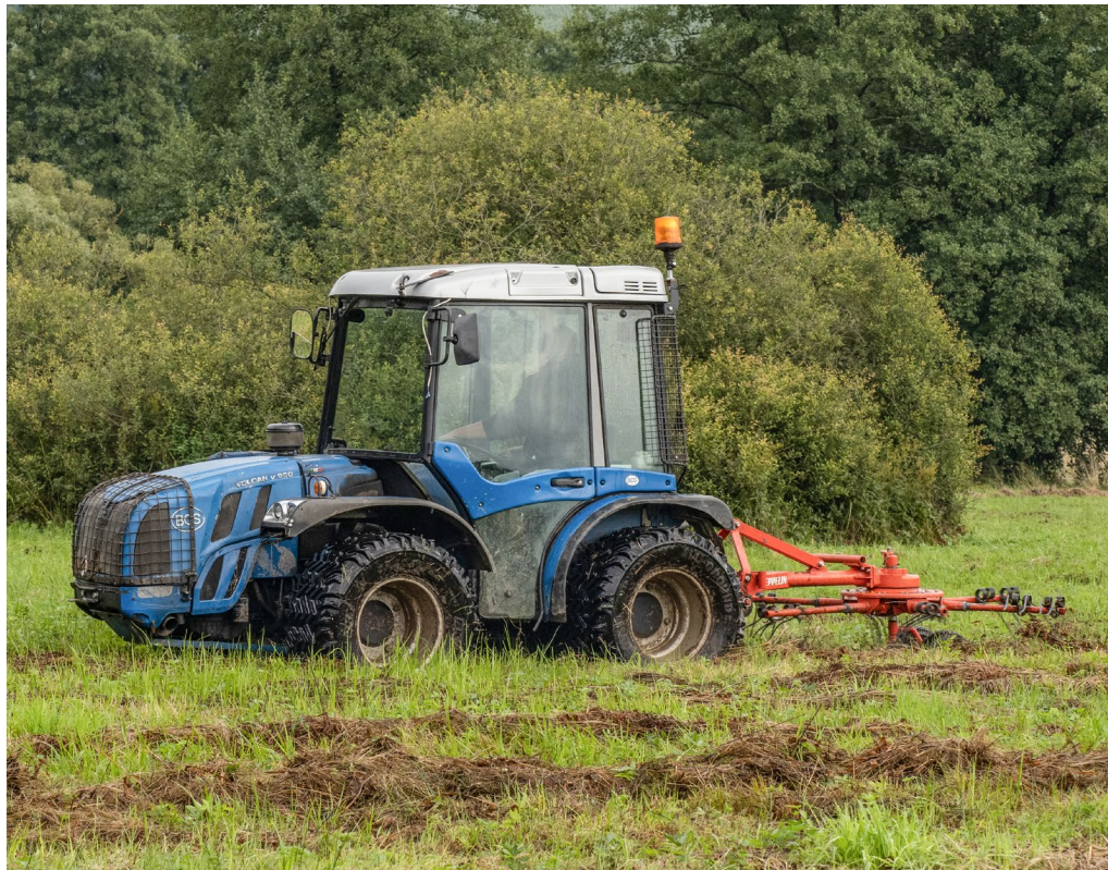
Figure 4. Example of a specialised small tractor with low-pressure tyres. © Václav Bystřický
